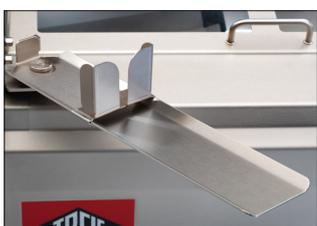
The bagging aid allows an easy and fast bagging of the sliced bread.
