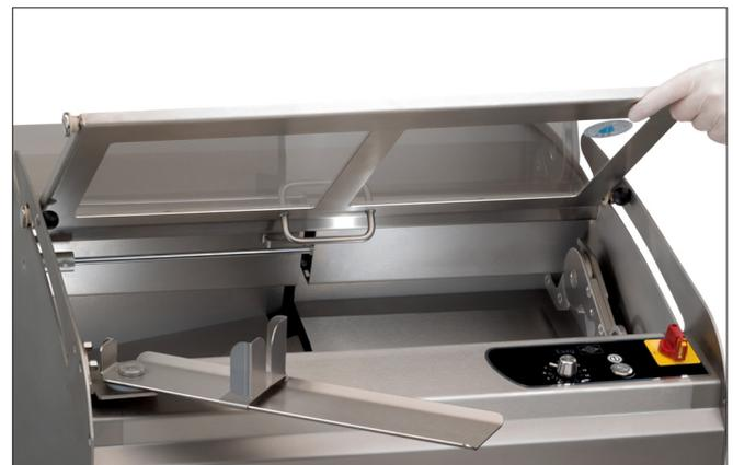
The Eazy is equipped with a moveable lid which can be wide opened so that the insertion tray is easily accessible for the cleaning process.
