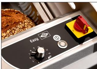
The high-quality operating panel makes the handling of the Eazy-bread slicer particularly easy and clear. As with the large series, you can set the cutting thickness via the rotary switch and start the slicing by pressing the button.
