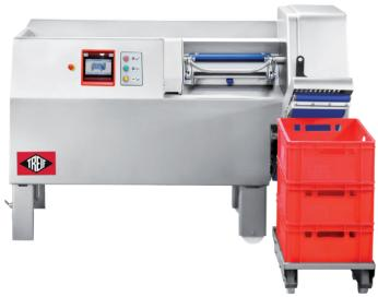
When equipped with the optional scale, ARGON+ stops as soon as the specified weight has been reached. Deviation from target weight is a maximum of +/- 0.3 %.
