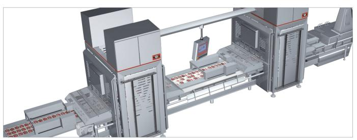
Different line solutions are possible, e.g. solutions with reduced personnel hours (Smartline) (belove) and the fully automated solution with robot technology (above).
