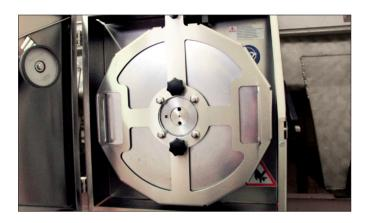
The sharpening devices are easy and safe to operate. The blade is assembled and disassembled with the help of a protection frame (as an example: HS divider orbital). On the HS divider and the HS divider orbital, a diamond-coated grinding tool provides best possible results.
