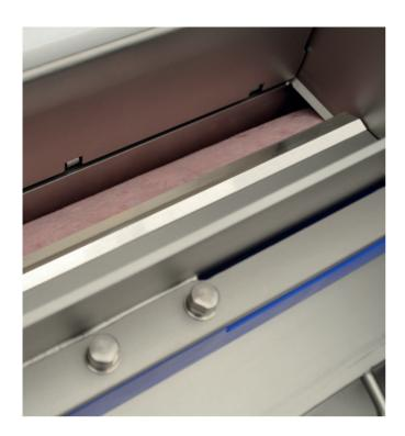
The separating slide operates in a curving motion. This is the only way to enable the convenient one-hand operation and fill the chamber to the maximum level.
